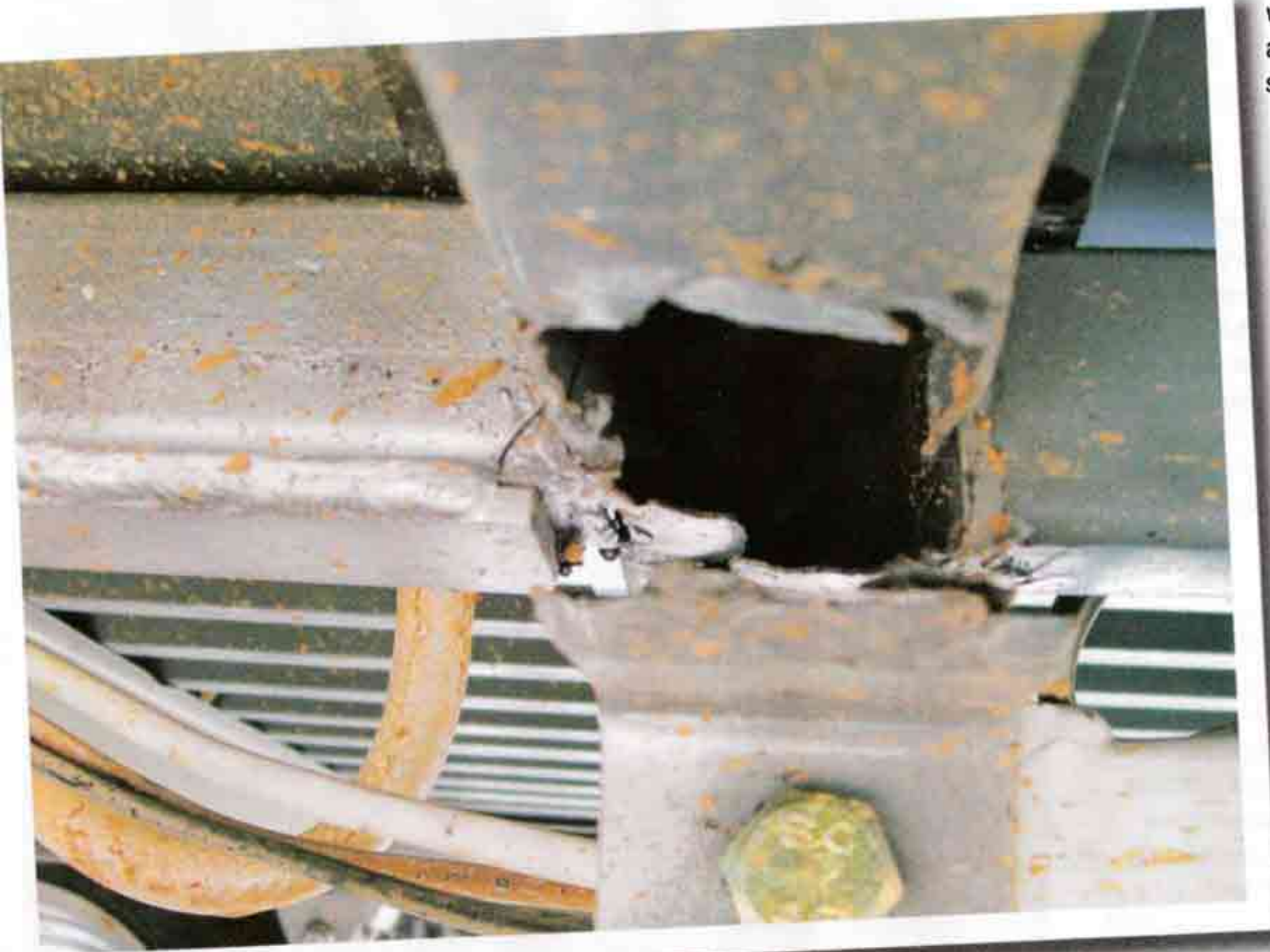
Above: Battery wiring should be neat, tidy and adequately protected – essentially the opposite to this...
