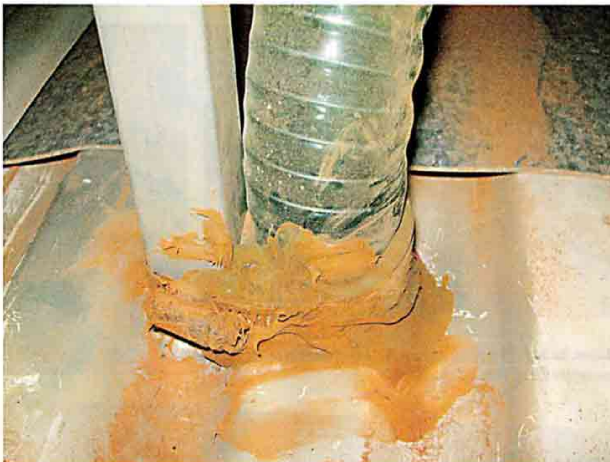
Above: A roadside repair, designed to keep some of the dust out of Jenny's trailer.
