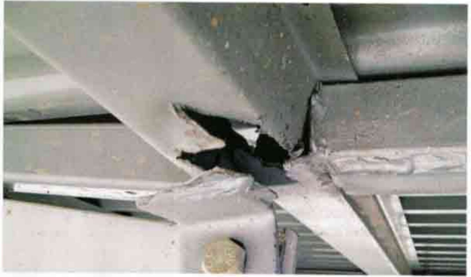
Above and left: It's a camper's worst nightmare: a cracked, and in this case completely separated, chassis.
